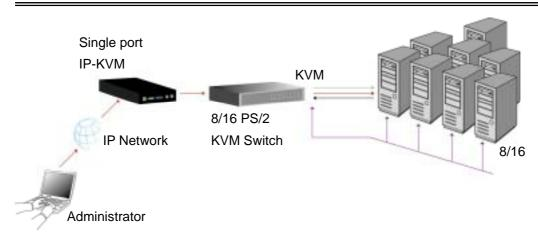
Figure 3-1.b: IP-KVM switch usage scenario
